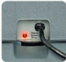
Carbon brush indicator lights red when brushes need to be replaced.
